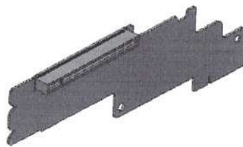
Figure 24. R3 Paddle (routes PCIe lanes to front backplane for additional NVMe)
