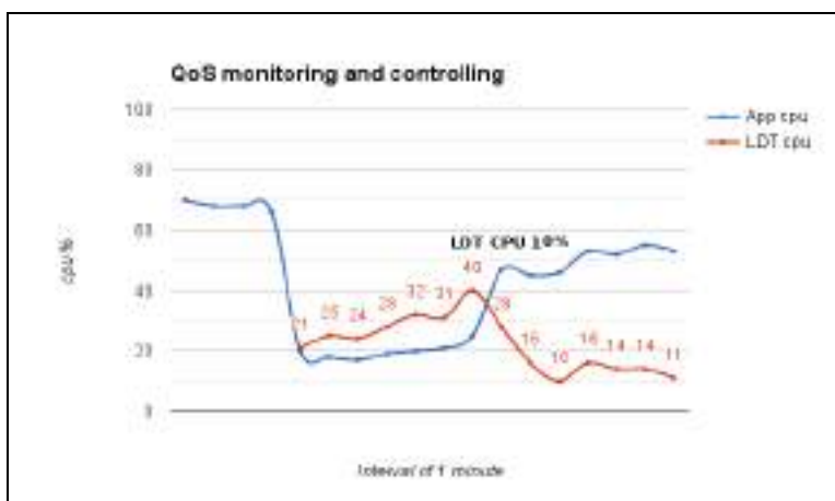
Figure 4-2: CPU usage allocation before and after QoS CPU parameter is set
